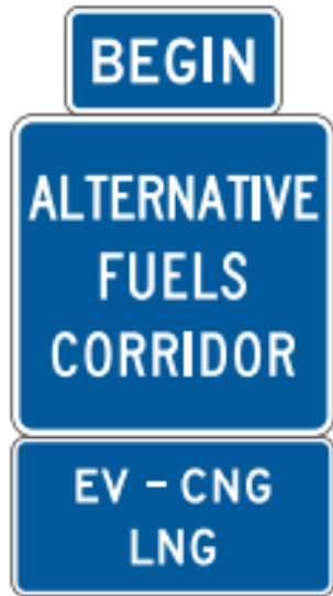
Alternative Fuel Corridor Signage (Section 2H.14)
